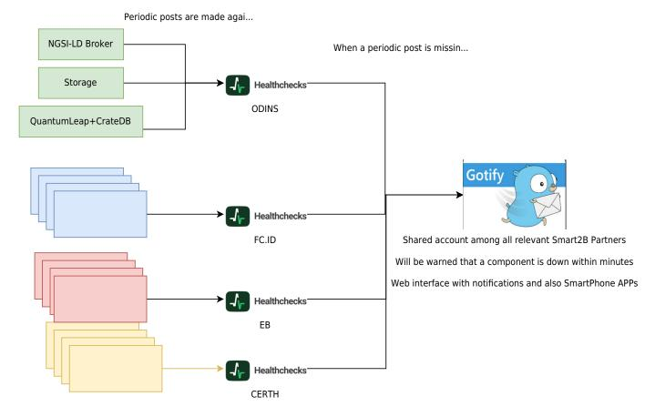
Due to the recent issues due to services being down in pilot tests, we will integrate a simple watchdog mechanism.
