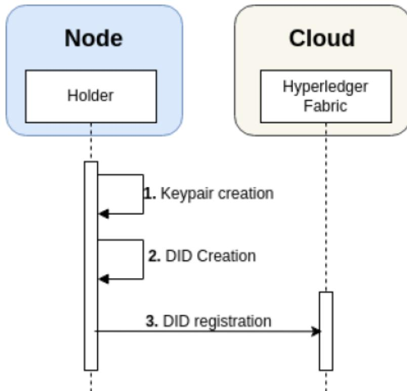
1. A key pair is generated using the ES256K algorithm. Both the public and private keys are stored locally within the Holder, specifically in the ‘data/key’ folder of each pod’s Holder. This folder, along with all directories under ‘/data,’ is created dynamically at runtime.
